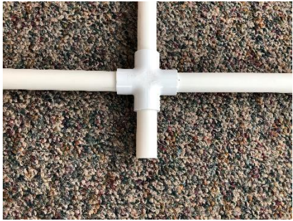
A cross fitting and short piping piece is used at the bottom of the Front Extender frame assembly.
