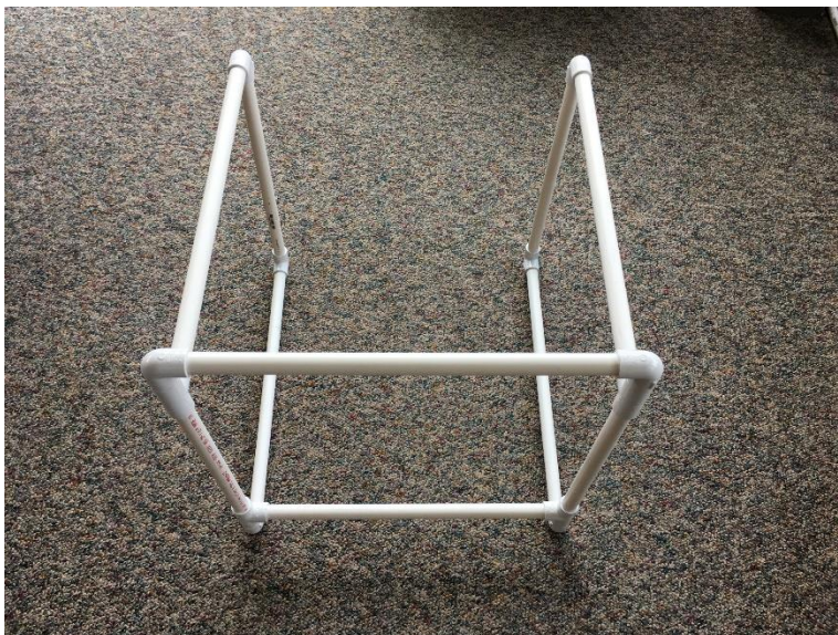
As you install the piping into the fittings, position the printing on the piping so that it will be covered by the panels, or otherwise not seen.
