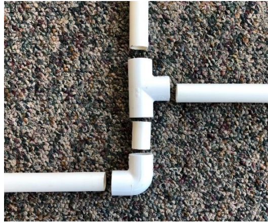
Assy & Exploded views right side lower tee joint (opposite side is symmetrical)
