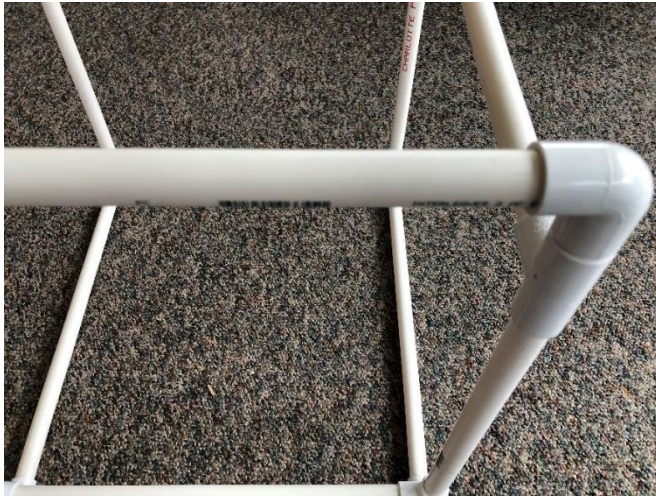
As you install the piping into the fittings, position the printing on the piping so that it will be covered by the panels, or otherwise not seen.
