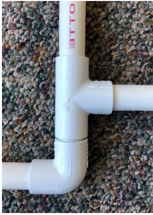
Assy & Exploded views right side lower tee joint (opposite side is symmetrical)
